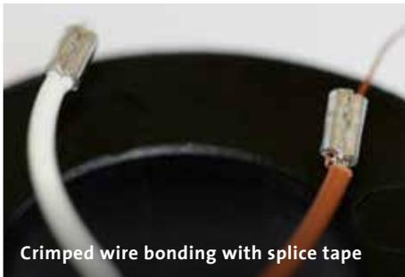
Crimped wire bonding with splice tape
